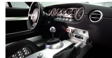
accentuated with the polished aluminum shifter and brake handle, along with the climate controls, audio system, starter button, and other switches. The gauges are traditional analog style and features a dominated oversized tachometer set in direct view of the driver, while the speedometer is offset to the right side.
