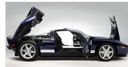
The rear clamshell engine cover is an aluminum shell hemmed to a carbon-fiber inner panel which helps stabilize the clamshell. The inner panel also
