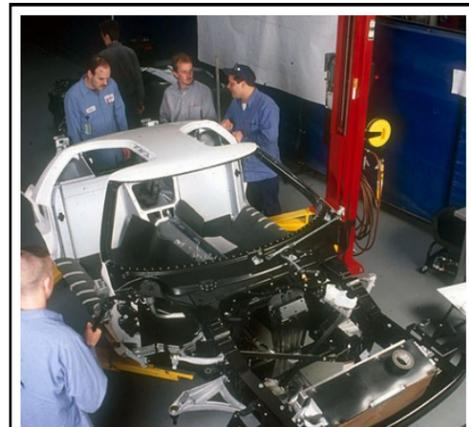
ABOVE: Chassis #1 arrives at the Ford GT shop, operated by Roush Industries, for the start of the major components installation. The suspension, powertrain, instrument panel, and seats all will be installed before final assembly takes place, including attachment of the body panels. Regular production of the Ford GT will take place at the Wixom Assembly Plant in Wixom, MI.
